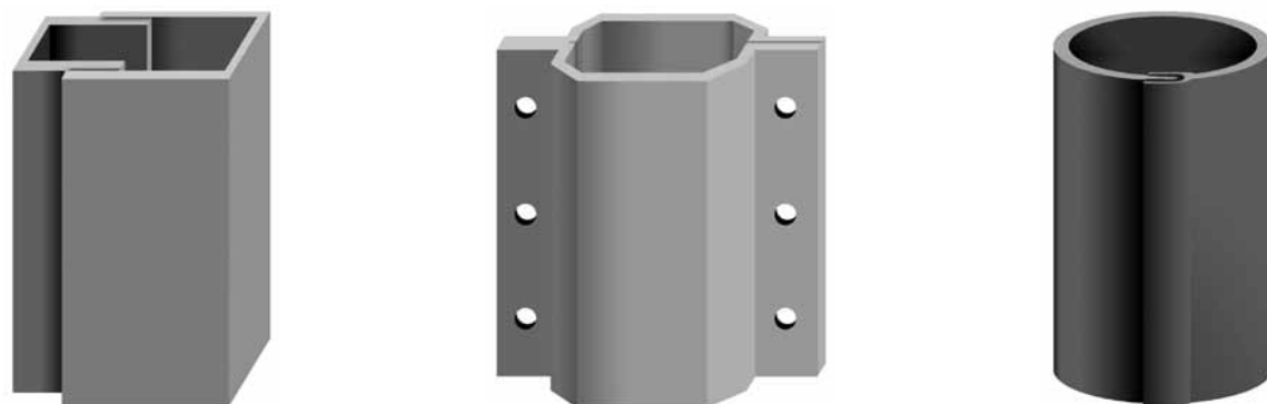
Fig. 1: Typical GFRP jackets used for repair of piles in North America
